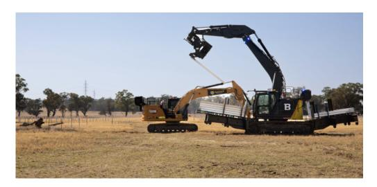
Bouygues Construction Australia (BCA), the Australian engineering, procurement and construction (EPC) arm of Bouygues Construction SA, is currently trialing an advanced Autonomous Piling System (APS) for the development of Engie's 250 MW Goorambat East Solar Farm (GESF) in Victoria, Australia.
