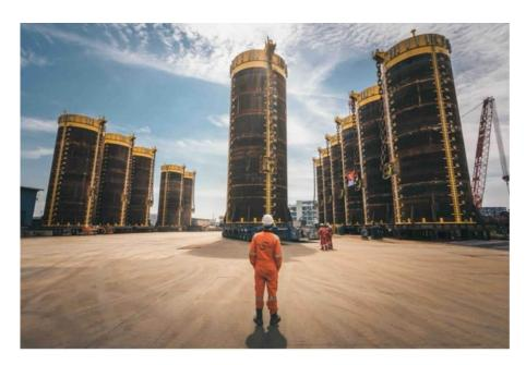
Franklin Offshore, a leading global provider of rigging and mooring equipment solutions and support to the energy industry, today announced that its wholly-owned subsidiary, CFE Engineers Asia Pte. Ltd (CFE Engineers), has successfully completed the fabrication and loadout of 12 gigantic suction piles for Chevron's high-profile Jansz-lo compression project offshore Western Australia.
